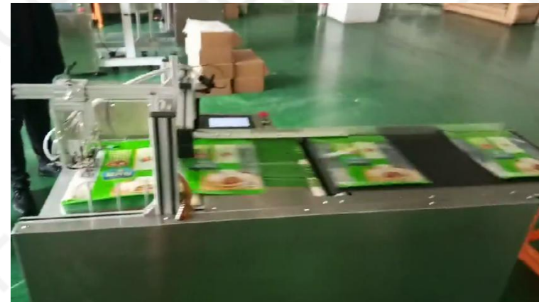
Paging machine with Prevent wrinkles function
