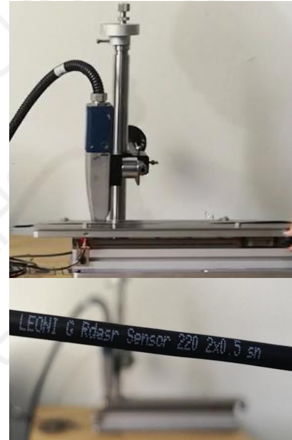
Printer equipped with sliding table ,print on tube
