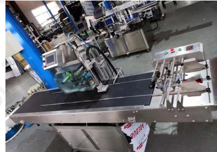
Paging machine with add tag function
