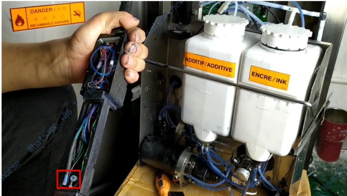
Then we can short-circuit the recovery valve here:
