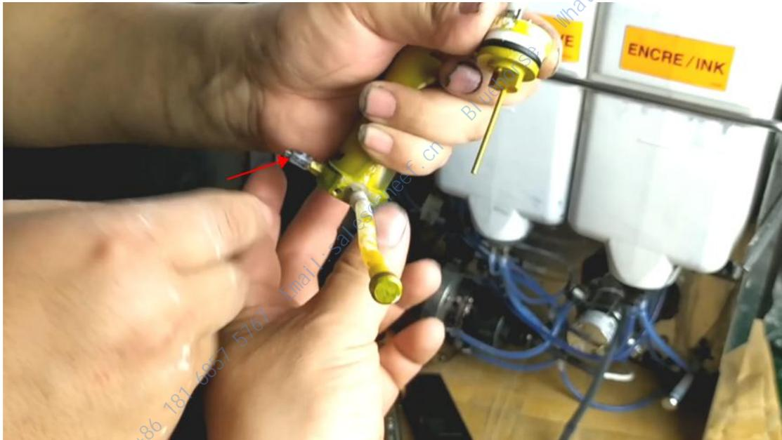
Then it continues to pump away after a period of time. If it finds that the viscosity is high in the process of extraction, the solvent adding valve will open, and then add solvent into it:
