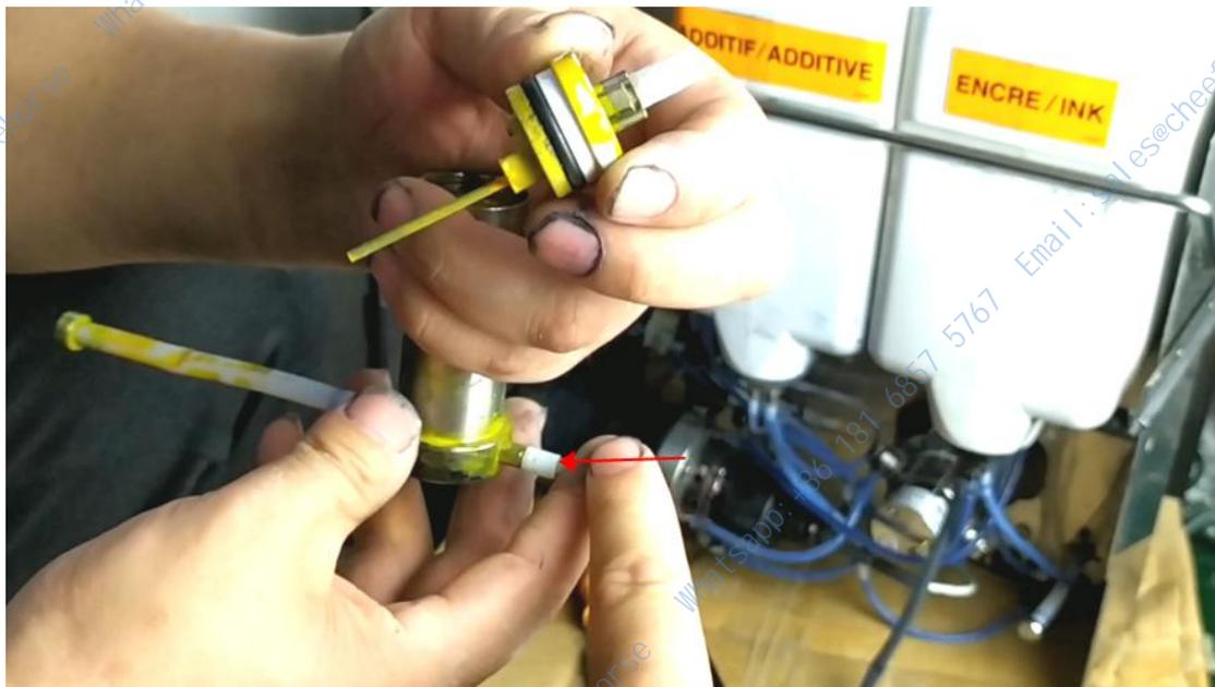
If there is no fault in your viscosity system, the viscosity will come out immediately. Then when it reaches the high level, the viscosity valve will open immediately, and the ink will be pumped out from this hole:
