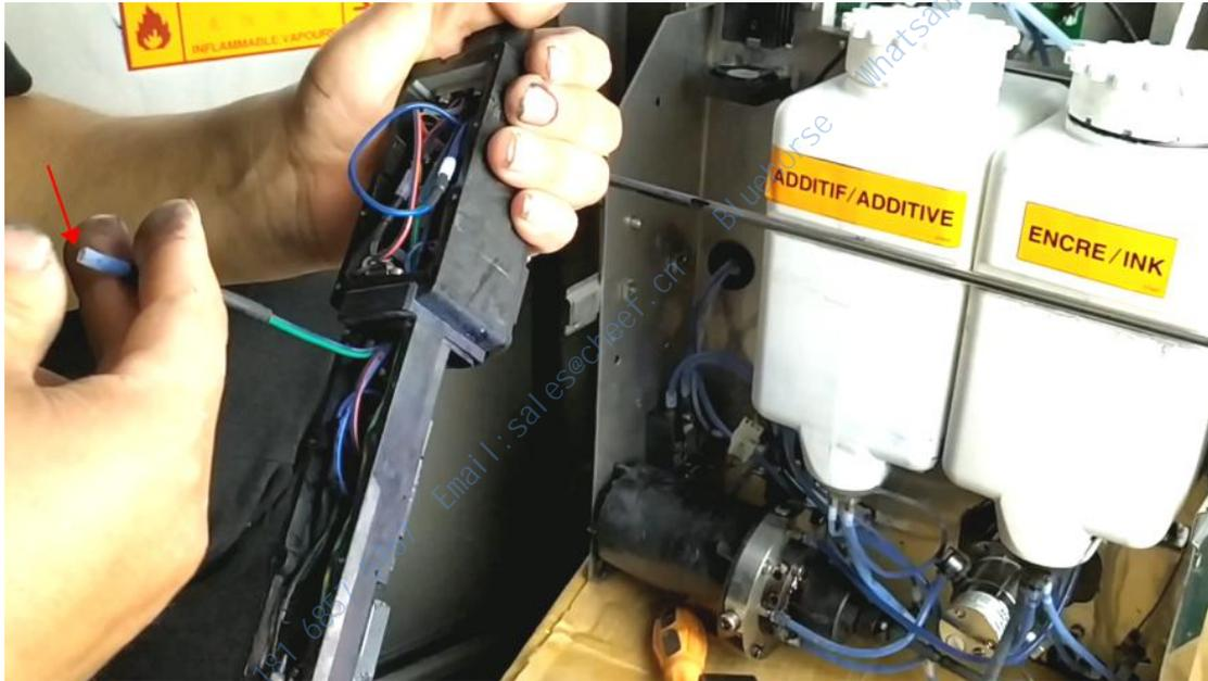
Blow hard. If the blockage is not very severe, use the ear ball to suck some cleaning solution to blow. Generally, it can be unobstructed.
