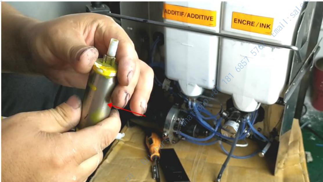
The viscosity of the machine that was repaired this time didn't come out. Finally, it was found that it was full of dry ink lumps after opening:
