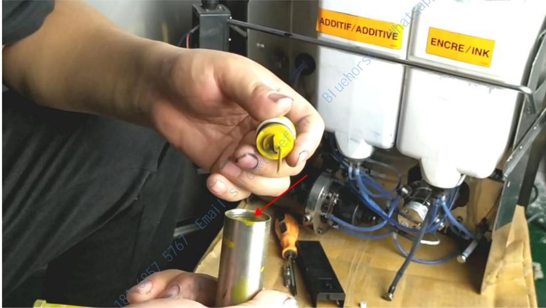
Although the pipeline is connected, it will affect the flow of ink and its detection, because it will feel that there is always ink, and then the viscosity valve will be continuously drawn out, and it will sound all the time.
