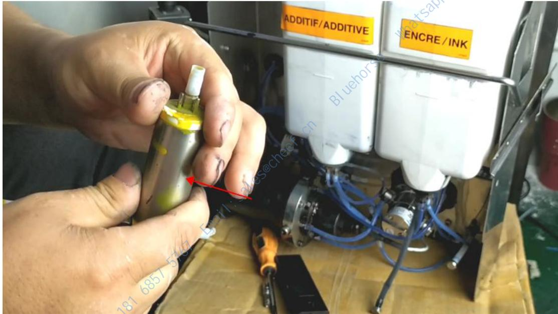
Normally, we first look at this viscometer to see if it is blocked, At the beginning, our direction was also wrong, because at the beginning of blowing from this side, all pipes were unblocked:
