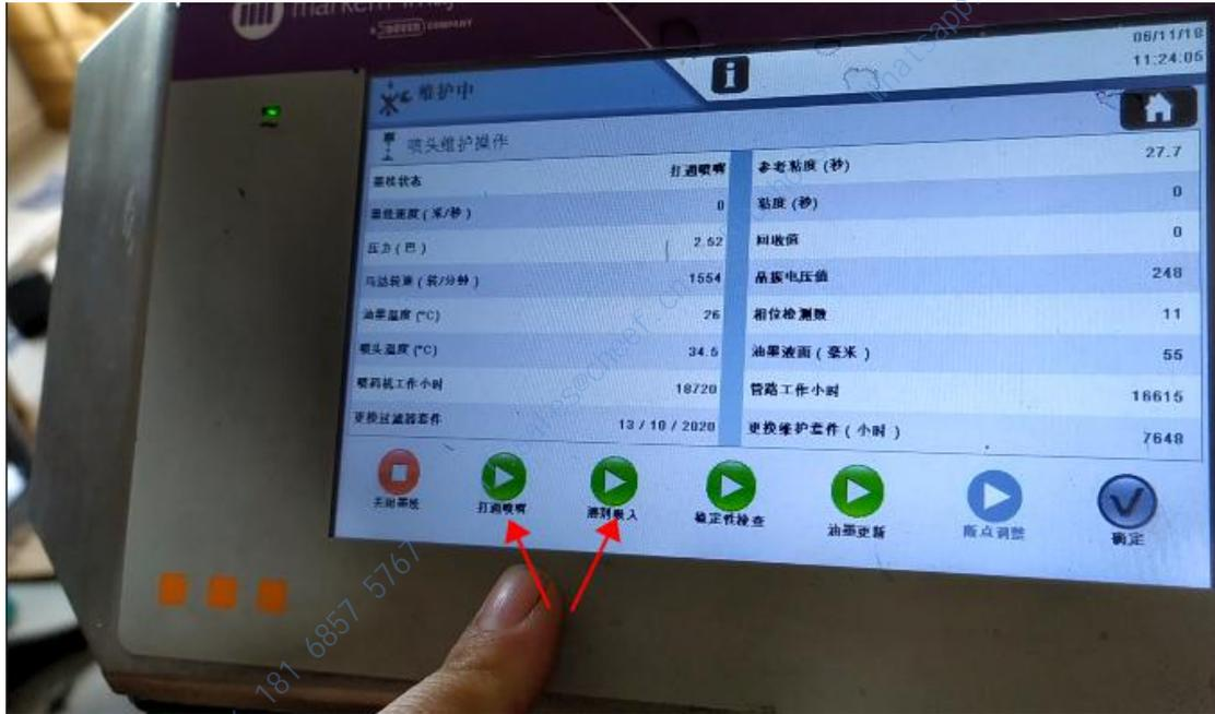
We can click on the "ink line stability check" to see the stability of the ink line, that is to say, hit the location of the recycling tank, whether jitter:
