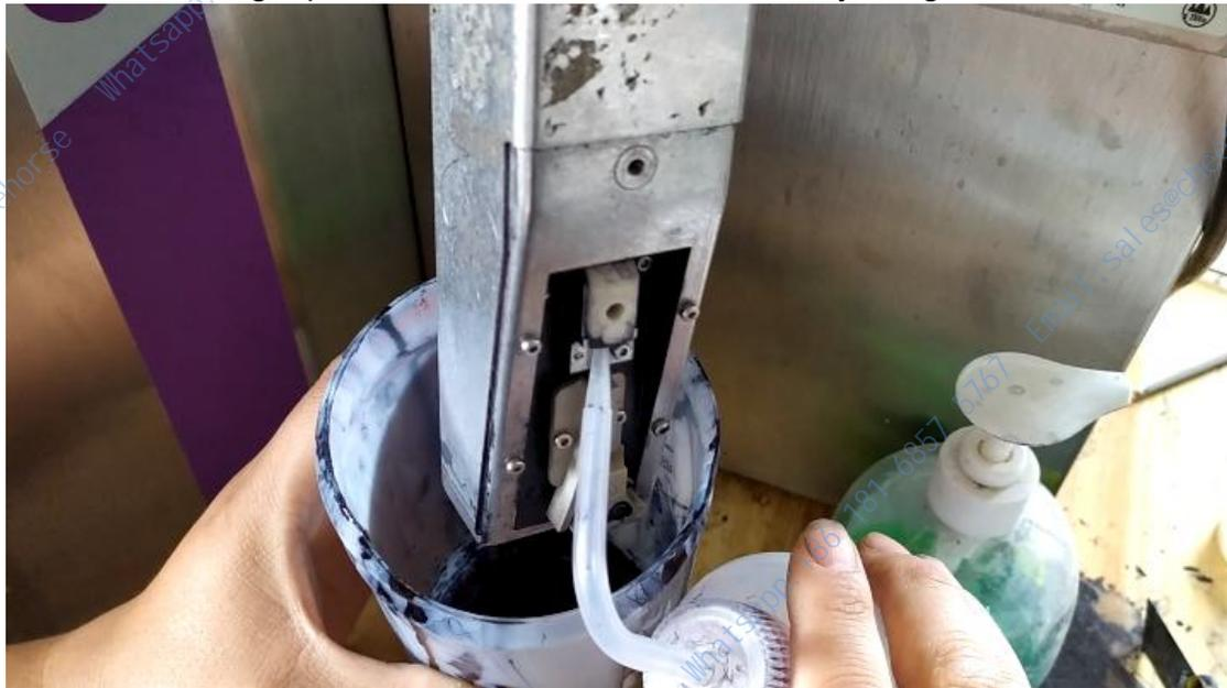
If the nozzle has not been opened, continue to open the nozzle, "Solvent suction" and "open nozzle" these two to cycle until the ink line is very stable:
