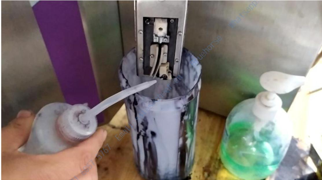
For example, recycling tank, as long as there is dirty place, you can wash it clean. Then, after washing, be sure to blow dry.
