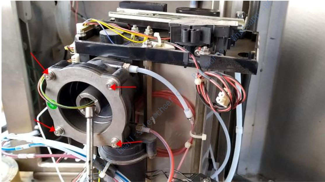
After removing the four screws, take this one out, and we will see the pressure sensor inside:
