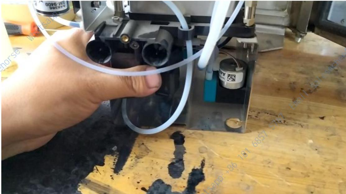
The measuring adapter is very easy to remove. We just need to remove this screw to remove the measuring adapter:
