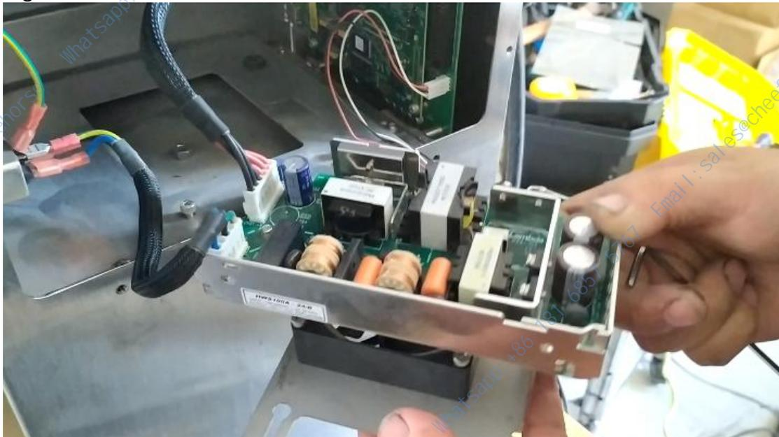
Now as soon as you pull the wires above it, the power supply is removed.
