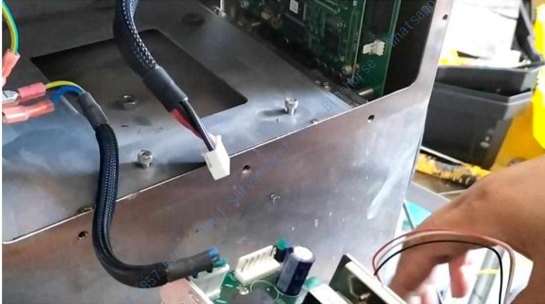
To remove the motherboard, we will loosen these two screws:
