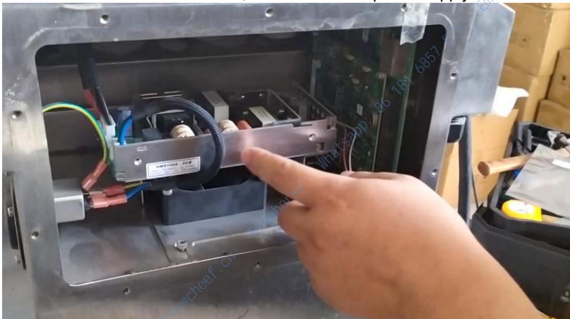
To remove the motherboard, we're going to take the two screws off:
