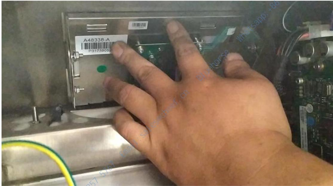
That is to say, if we want to remove this, the front panel needs to be removed, otherwise we can't push it from the back.
