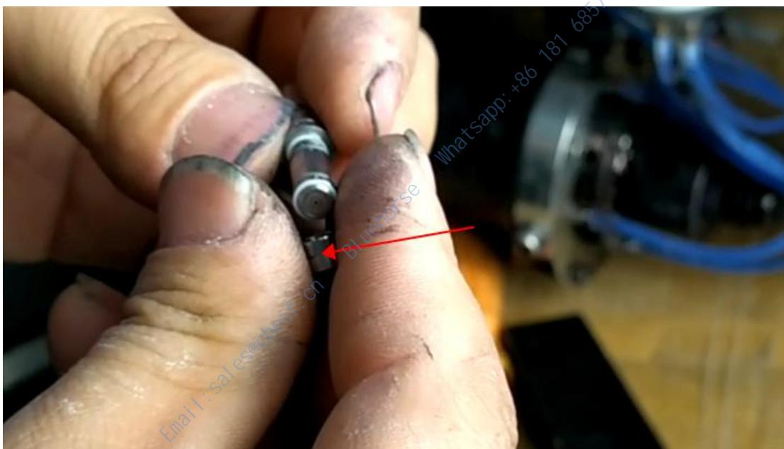
Then remove the white O-ring at the back. Don't lose the O-ring:
