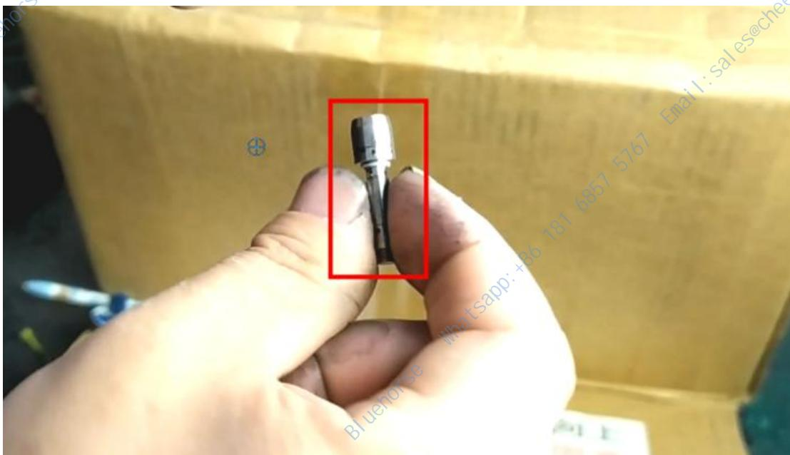
In general, if ultrasonic cleaning is used, we should put it vertically upward in the ultrasonic wave. In this way, if there is something dirty, it will enter below:
