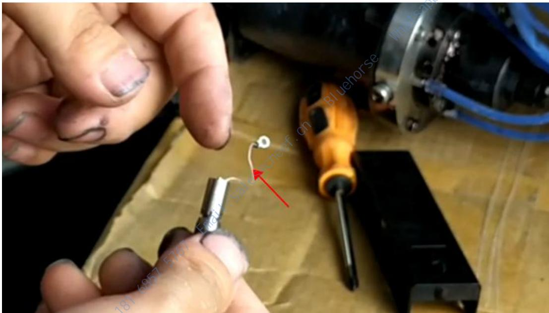
After we put it on, we directly use "nozzle to punch through", and see if the ink line is out or it is originally without ink line. Now that there is ink line, we will see the position of the ink line is right. If the position of the ink line is OK, it is straight, not slanting, then we can install it.
