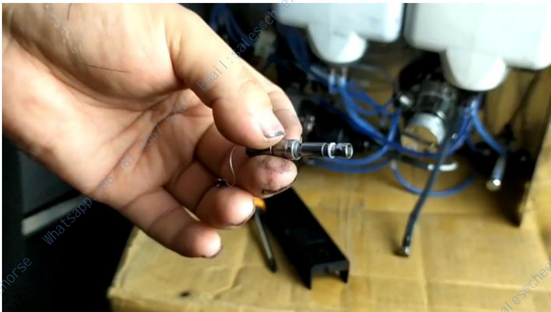
Then put it directly into the ultrasonic wave for cleaning, but don't use heating, just put it in it and let it vibrate. After the vibration, as long as it's not blocked, it's generally OK. However, it may not work if the blockage is very, very severe, but under normal circumstances, the quick solution is to use ultrasonic to clean it without dismantling it, so as to prevent the loss of its accessories.
