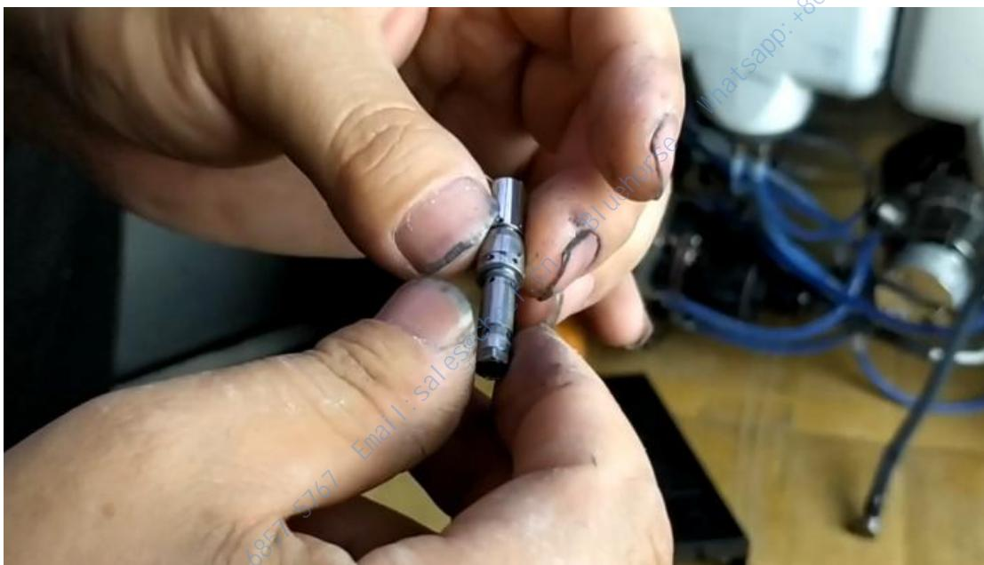
After we screw the screw off the back, this is the nozzle:
