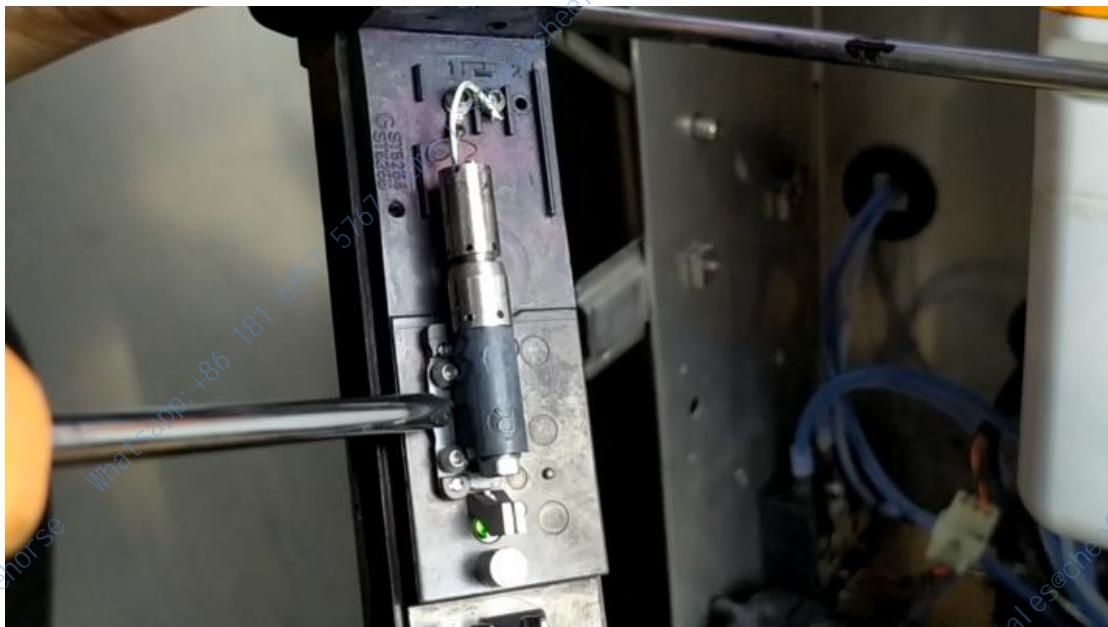
If you want to remove the nozzle, let's loosen the two screws first. One is the ground wire and the other is the crystal oscillator wire. Let's loosen them first:
