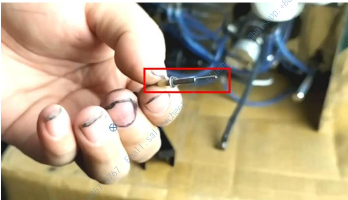
If the crystal oscillator is dirty, we can clean it, but don't use ultrasonic cleaning, otherwise the O-ring on it will be broken.
