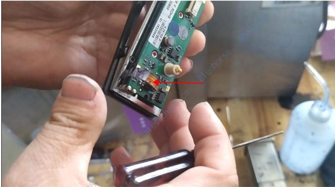
This row is directly connected to the recycling tank, if you want to remove the recycling tank, first remove this row, and then loosen the screw, and then pull the recycling tank out:
