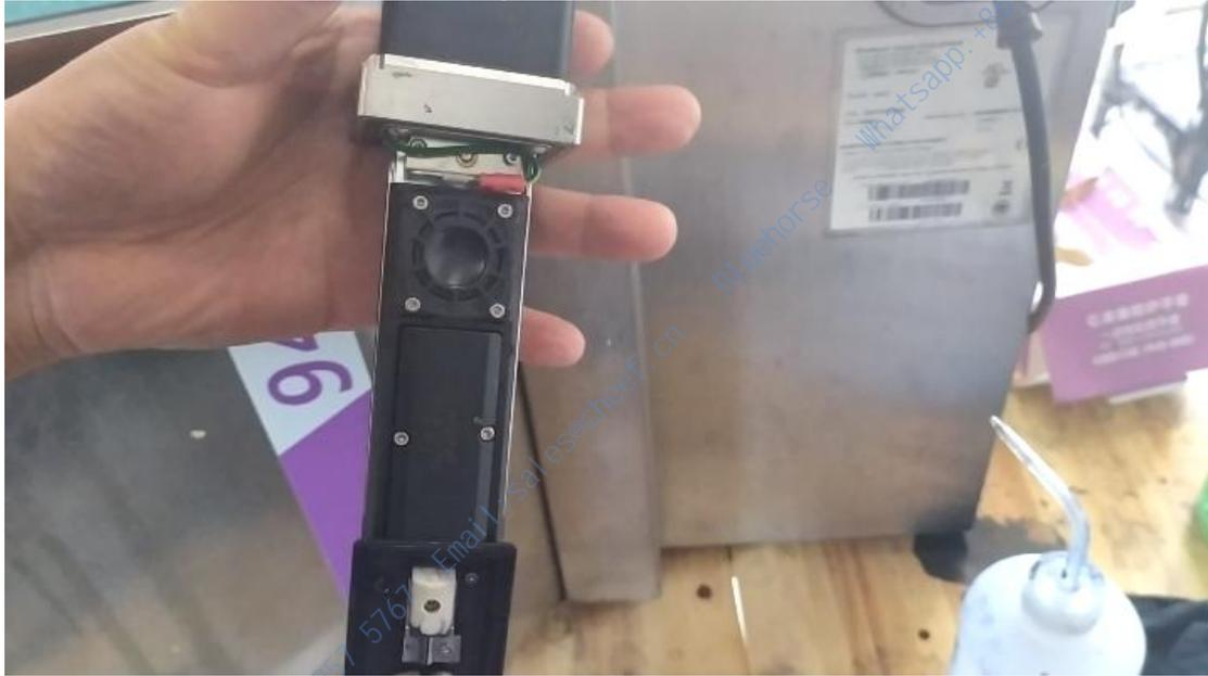
There is a nozzle solenoid valve here, if we want to remove it, put it on top of two screws can be removed as soon as it is loose:
