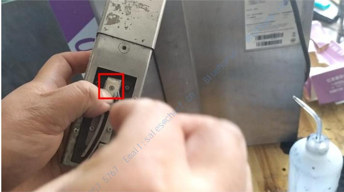
If you want to remove the recycling tank, first unplug the line on the rear sprinkler board, then remove the screw, and then pull the recycling tank out:
