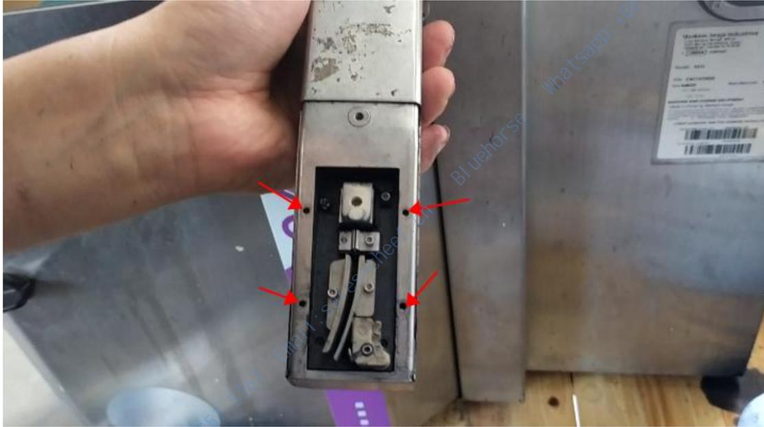
If you want to replace the charging slot, also loosen the screw:
