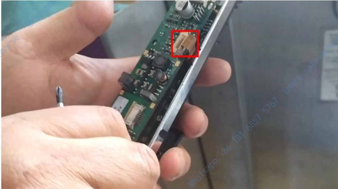
Then, after unplugging the top row, the board can be removed:
