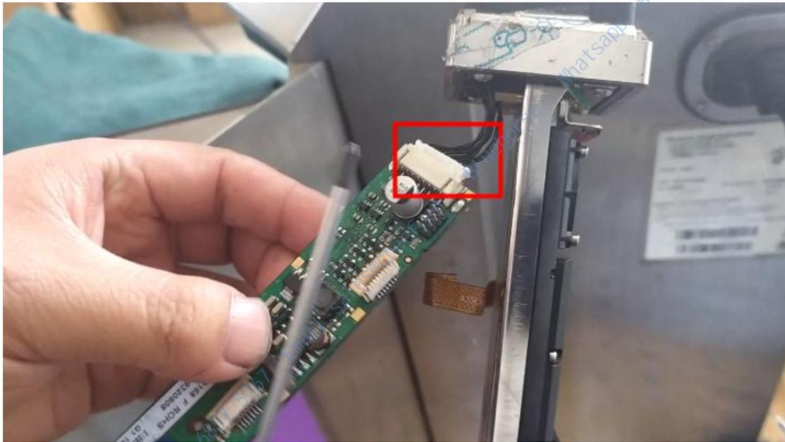
When installing the circuit board, install two screws to secure it:
