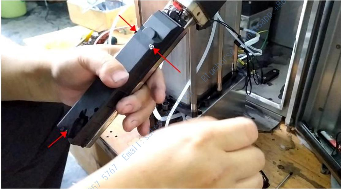
Then we install the solenoid valve. The solenoid valve can be divided into positive and negative parts. The electrified part and the board should be put together:
