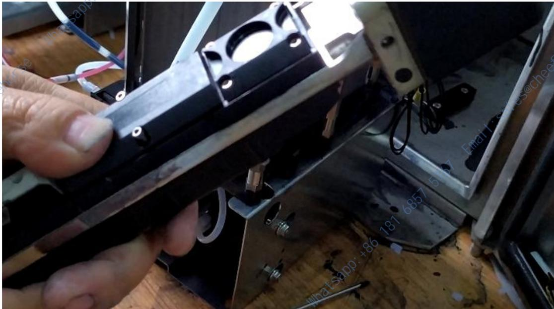
Let's see how the nozzle is removed, just loosen the screw and the nozzle can be removed:
