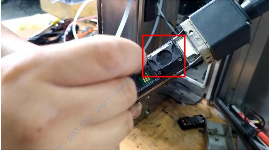
Then the nozzle filter can be removed:
