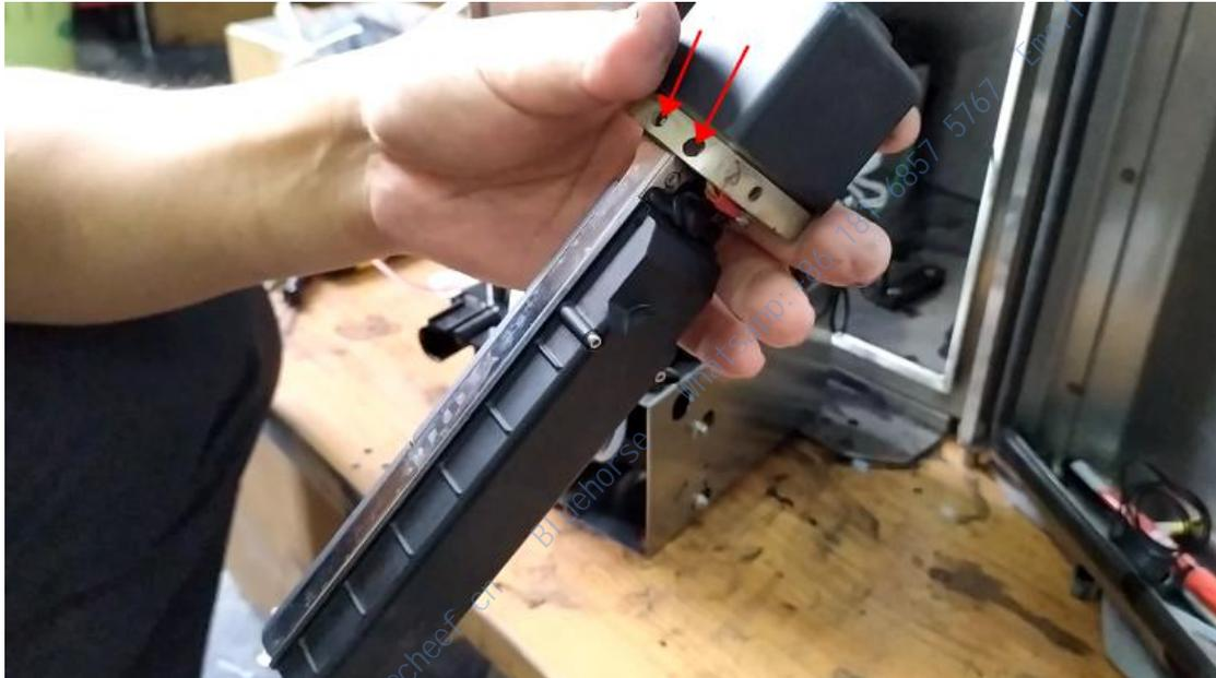
Then first we remove the solenoid valve:
