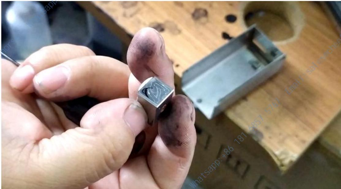
Get it stuck, then tighten the screw and the nozzle is installed:
