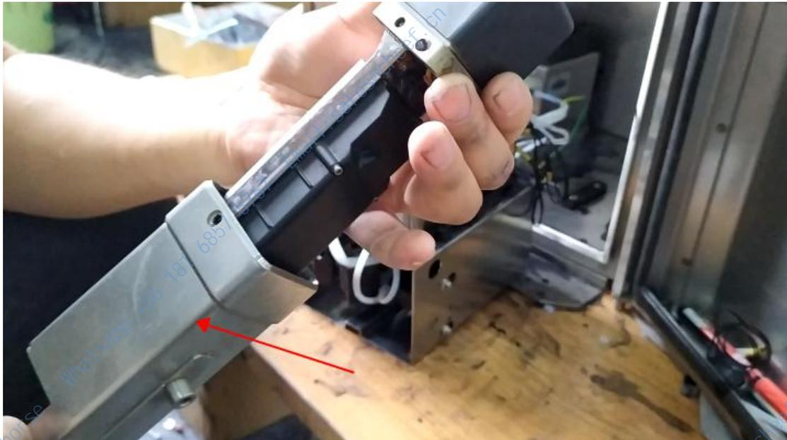
There are two screws on it. After removal, the cover can be directly removed:
