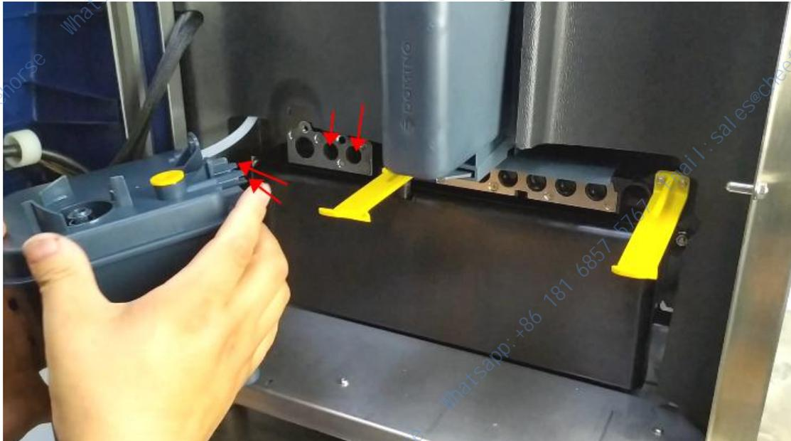
Then we insert it in, and we must firmly plug it in, because if the two holes and sealing rings are not firmly inserted, air will leak:
