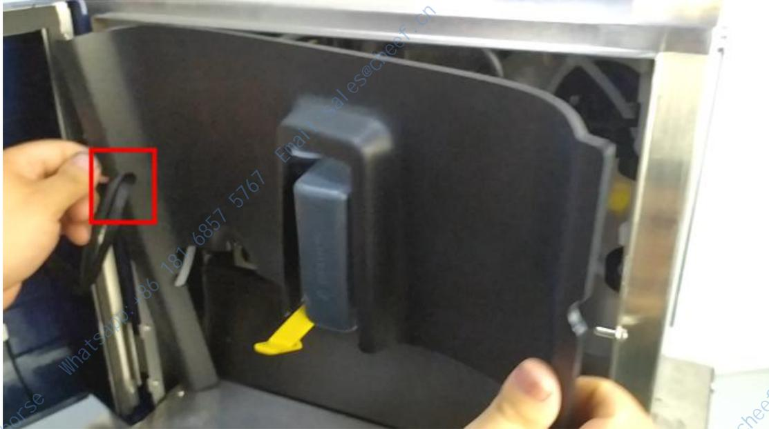
Then, the baffle installation is completed:
