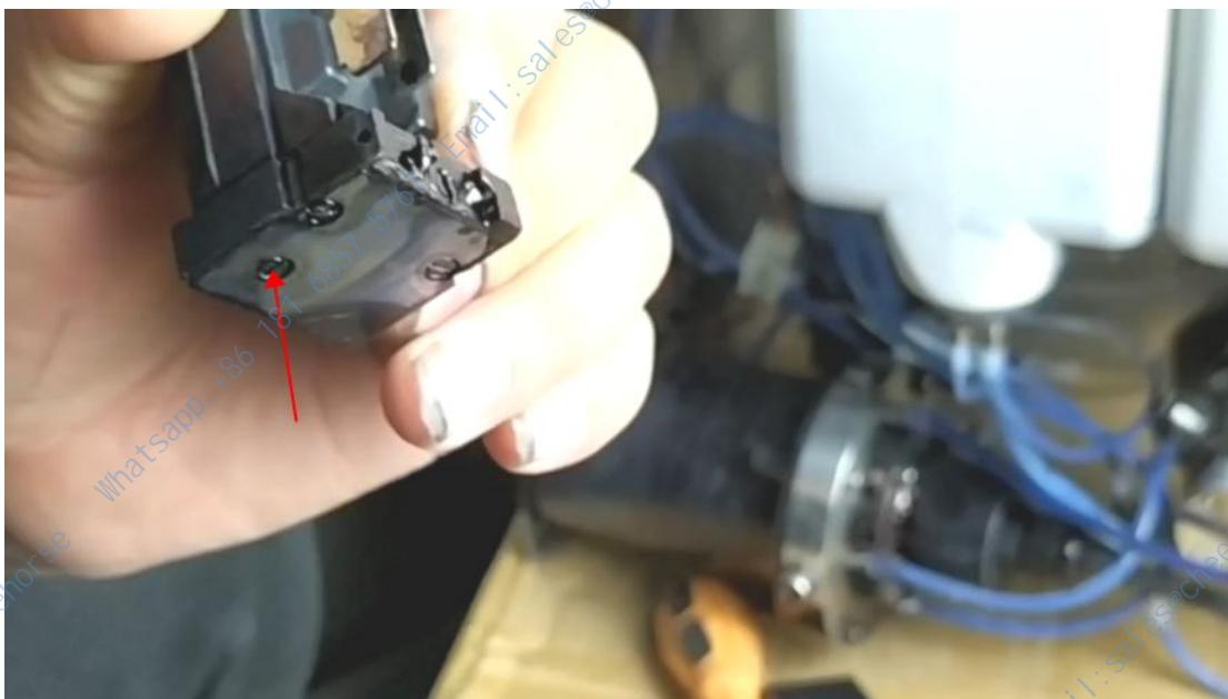
But when dismantling, we should pay attention to the fact that there are three very small O-rings around the column. Do not remove the O-ring. If it is removed, even if we screw it tightly, it will leak ink. We need to pay special attention to this.
