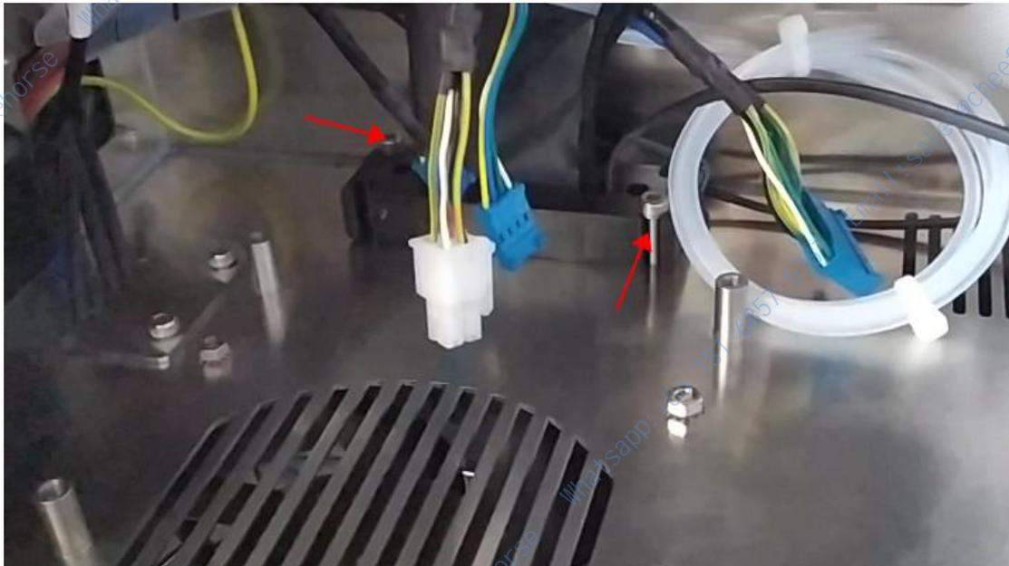
If the screws are not easy to install, we can first remove the motherboard, we remember how the lines on the motherboard are installed, and then remove the motherboard, so that the operation will be very simple.
