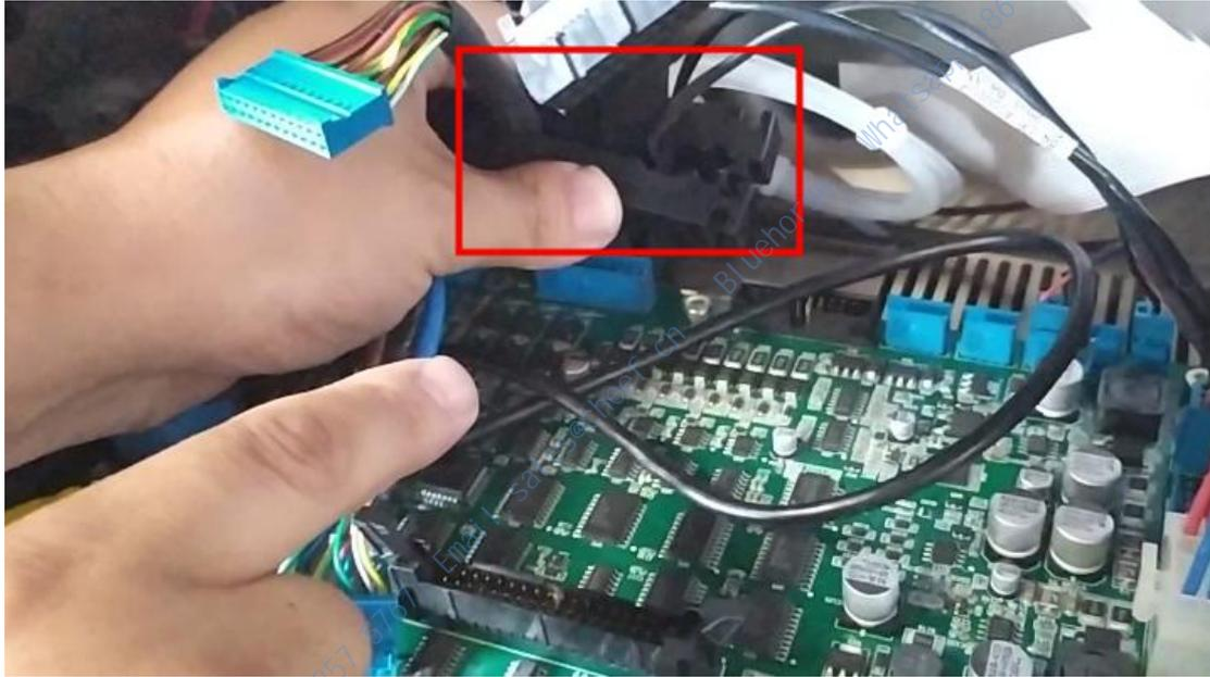
This fixed block, the line to wear in. It can be dislocation, this is two pieces, it is stuck together, we do not use brute force to force them apart. We need one finger up, one finger down, stagger them like this, and this fixed block can be removed:
