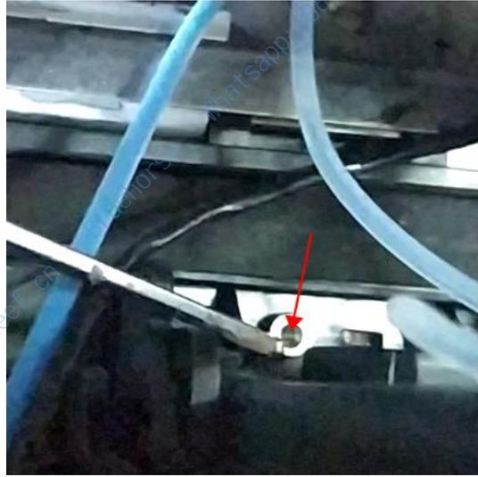
There are two screws at the front and back of the ink box slot and the solvent box slot. When removing, remove the two screws at the front and back respectively.
