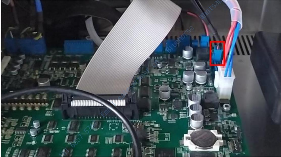
In particular, it is important to remove the wire before removing the ink box slot and solvent box slot. If you remove the wire, first unplug it:
