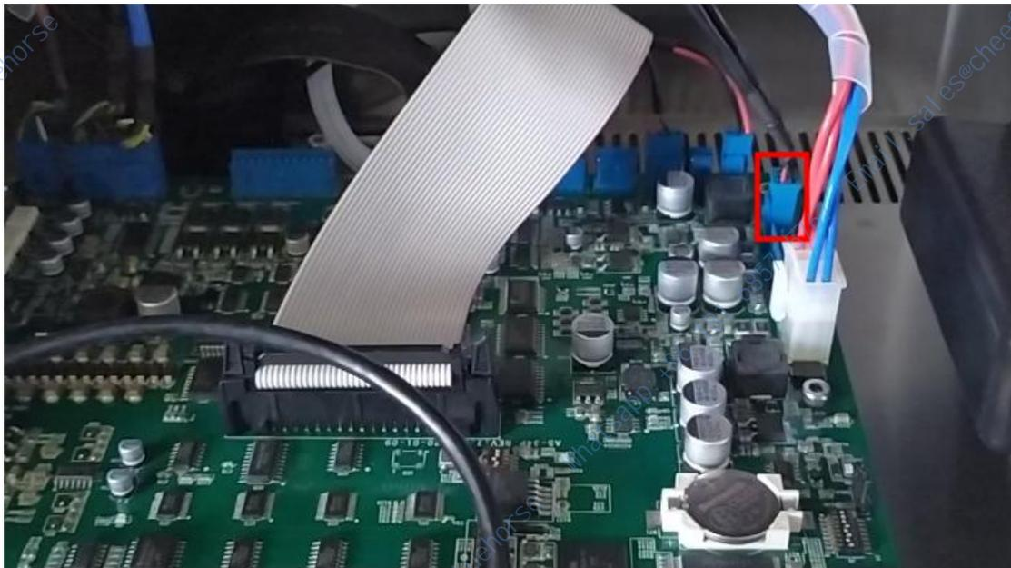
After pulling it out, because the cable is connected to the black fixing block, if it is difficult to remove, we need to remove the motherboard first, and then remove the two diagonal screws of the black fixing block, and then we need to stagger the black fixing block up and down. After staggering it, the cable head can be removed from below:
