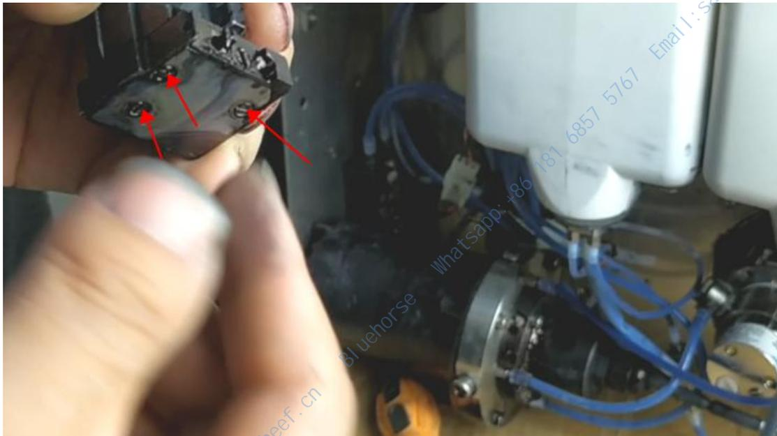
Then up and down, we can use a slotted screwdriver to raise the stainless steel rod up a little, and we can also fine tune it left and right a little:
